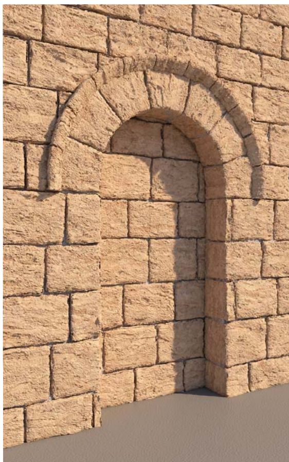
Fig. 6-4. Visualization of the elements of a hoodmold above a niche
