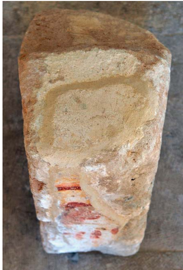
Angled view, showing the concavity in the intrados surface and the large loss on the back of the stone
