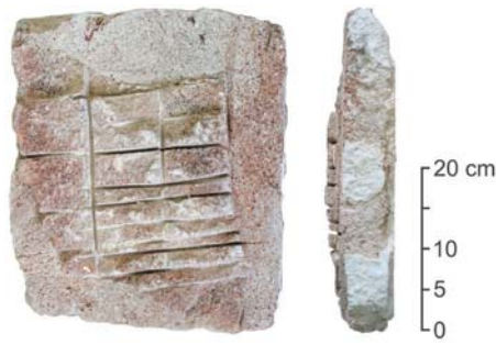
Fig. 4-2. The back (left) and one of the sides (right) of ashlar Cat. 30d showing deep cuts made with an angle grinder
