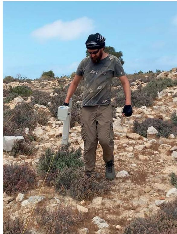
Fig. 4. Survey with fluxgate gradiometer Geoscan Research FM256 (photo T. Herbich)
