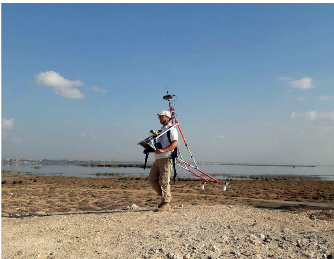
**Fig. 5.** Survey with the Geometrics G-858 caesium magnetometer and SH3 Topcon Real Time Kinematic Global Positioning System (photo K. Misiewicz)
